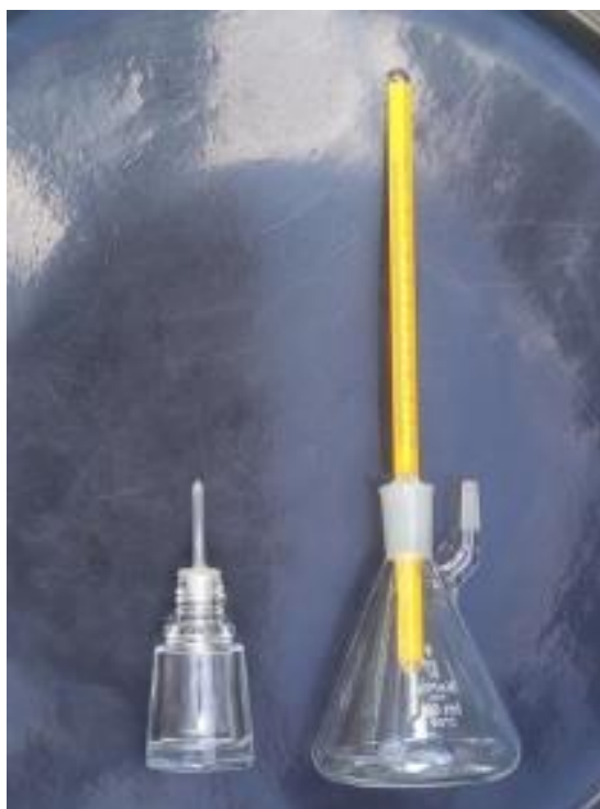
Figure 4. Improvised pycnometer (left) and standard pycnometer (right).
