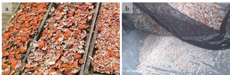
Figure 1. Crab shells before and after grinding. a) Sun dried crab shells, and b) Pulverized crab shells.
