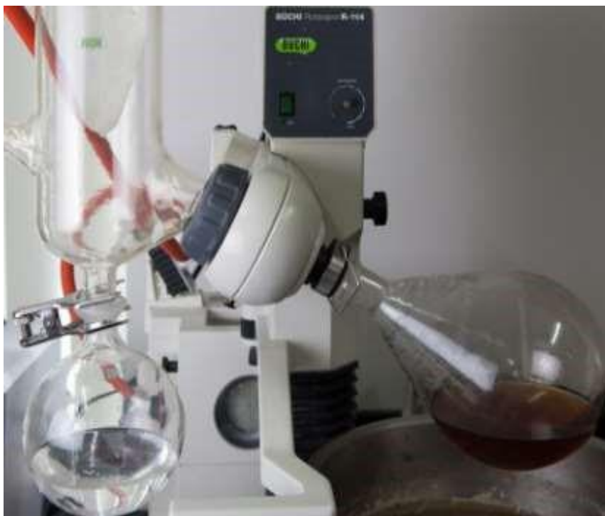
Figure 2. Sappan seed ethanol extract (SSEE) in rotary evaporator.
